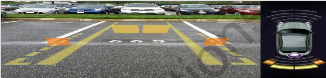
☞ Change the size of image : Press **CAM button** in Rear mode.
